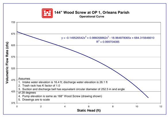
Operational Curve for 144" Wood Screw Pump at OP 1
