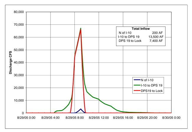
Figure 2-17. Calculated Flow Through and Over Inner Harbor Navigation Canal Floodwalls. Based on Preliminary ADCIRC Hydrographs Adjusted Using Gage Data from IHNC Lock
