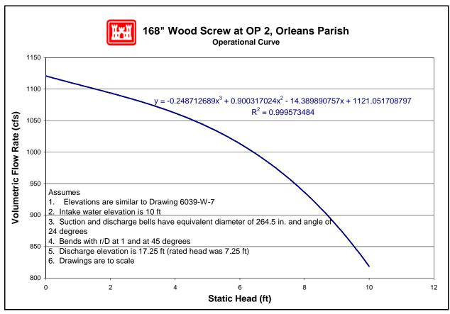
Curve for 168" Wood Screw Pump at OP 2
