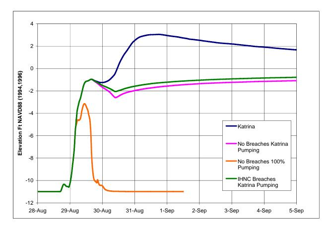
Figure 2-22. Calculated Water-Surface Elevations in Storage Area 14
