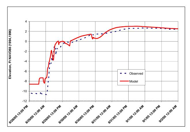
Figure 2-11. Calculated and Measured Stages on the Palmetto Canal at Jeff Davis Parkway During Katrina
