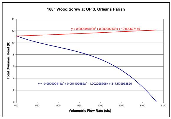
System Curve of 168" Wood Screw Pump at OP 3
