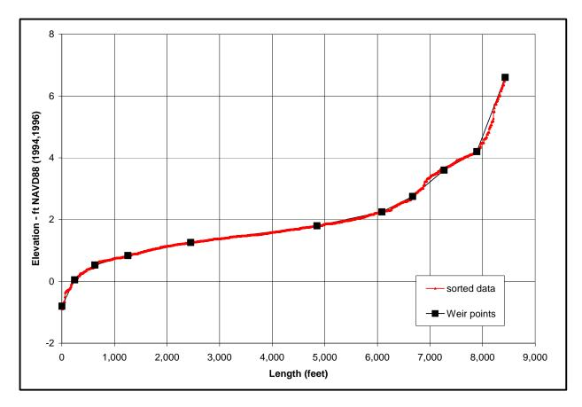
Figure 2-8. Sorted Weir Profile Between Storage Areas E3-16 and E3-17 Pumping Stations
