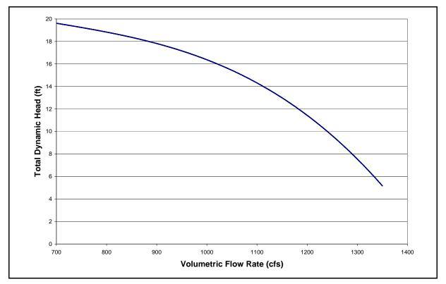
Figure 7-13 – Typical Pump Curve
