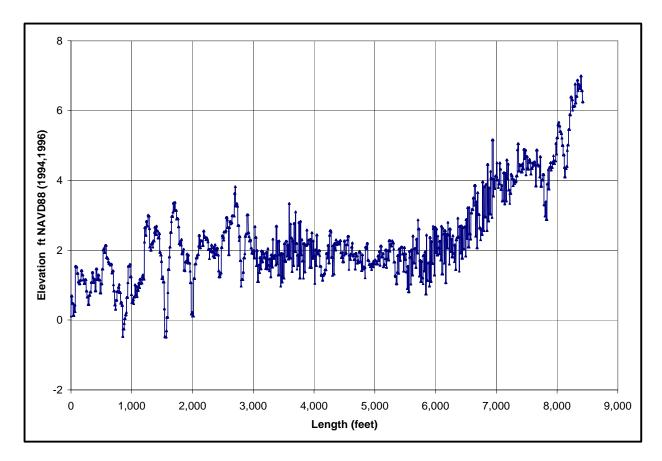
Figure 2-7. Digitized Weir Profile Between Storage Areas E3-16 and E3-17
