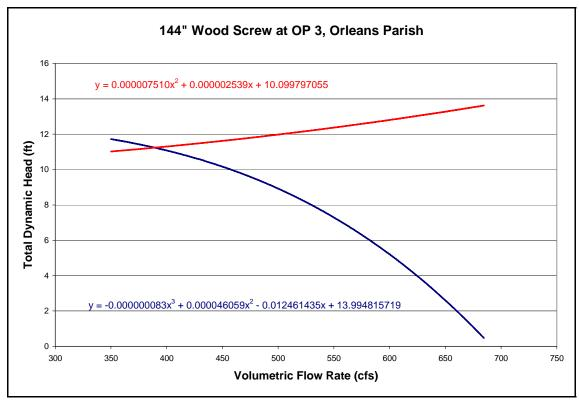
System Curve of 144" Wood Screw Pump at OP 3
