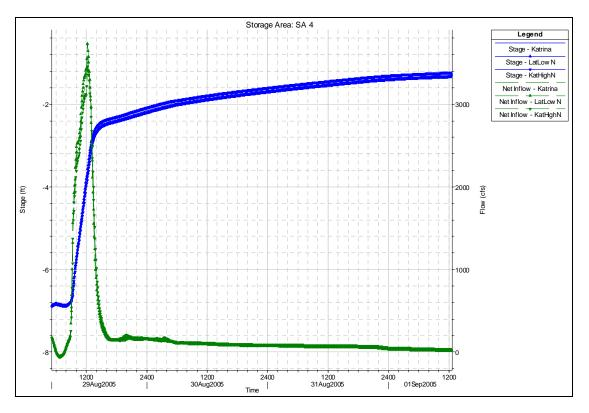
Figure 6-21. Computed Stage and Flow for Storage Area SA 4
