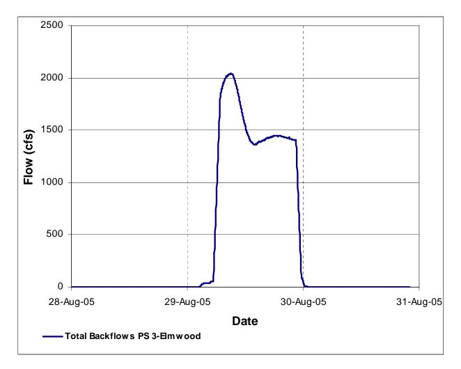
Figure 1-12. Estimated Backflow Hydrograph, East Bank, Elmwood Pump Station
