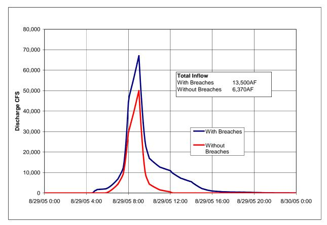
Figure 2-18. Comparison of Calculated Flow at IHNC Floodwall Between I-10 and Pumping Station 19 With and Without Breaches During Hurricane Katrina. Based on Preliminary ADCIRC Hydrographs Adjusted Using Gage Data from IHNC Lock.
