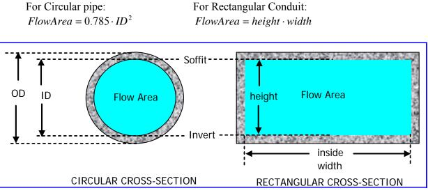
Figure 7-21 - Geometry Terms and Dimensions for Circular and Rectangular Conduits
