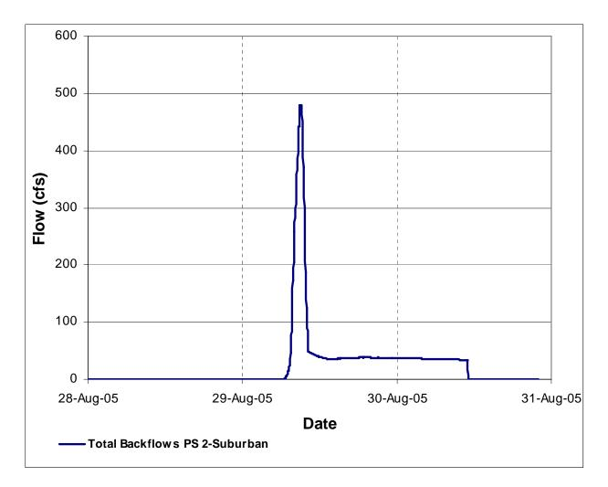
Figure 1-11. Estimated Backflow Hydrograph, East Bank, Suburban Pump Station
