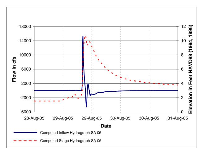
Figure 4-10. Computed Stage and Flow Hydrographs for Storage Area 05 for Katrina Simulation
