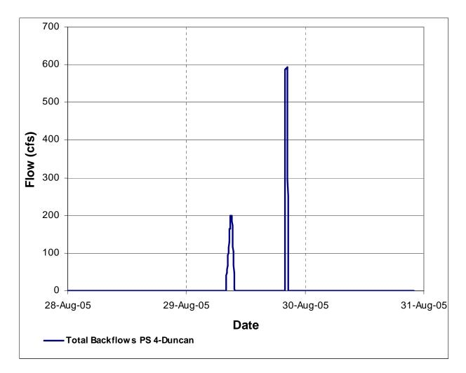
Figure 1-13. Estimated Backflow Hydrographs, East Bank, Duncan Pump Station
