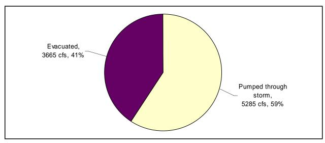
As shown in Figure 7-10, 59% of the parish's West Bank rated pump capacity was not evacuated and pumped during the storm.
