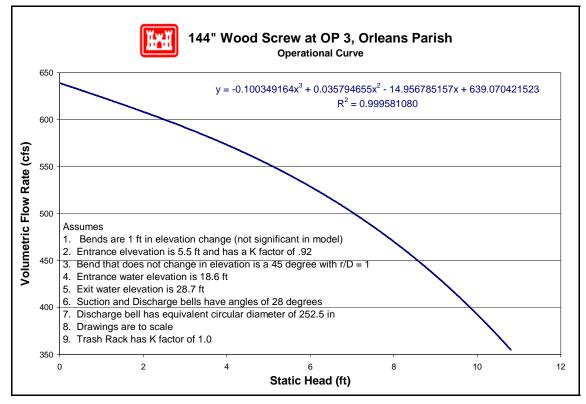
Operational Curve for 144" Wood Screw Pump at OP 3
