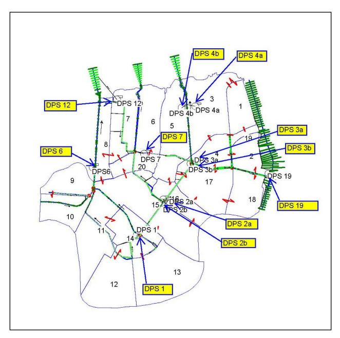
Figure 2-9. Pump Stations Modeled in HEC-RAS Model
