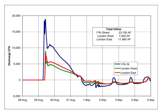
Figure 2-16. Calculated Flow Through Levee Breaches. Based on Observed Stage Hydrographs
