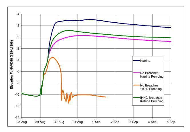
Figure 2-20. Calculated Water-Surface Elevations in Storage Area 5
