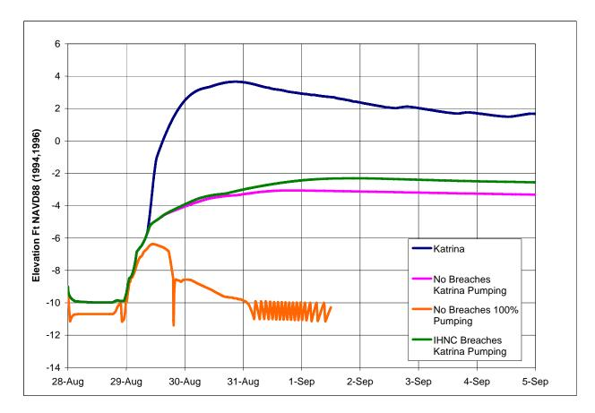
Figure 2-21. Calculated Water-Surface Elevations in Storage Area 7
