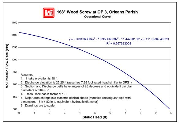
Curve for 168" Wood Screw Pump at OP 3
