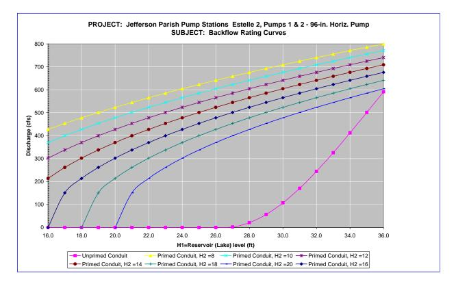
at the soffit of the crest pipe drops below -9.5 psi gage pressure. Either case is a siphon breaker.
