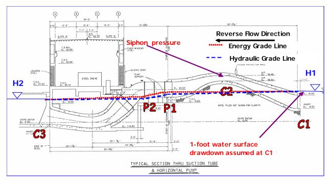
Figure 7-26 - Locations Where Siphon Flow Can be Broken
