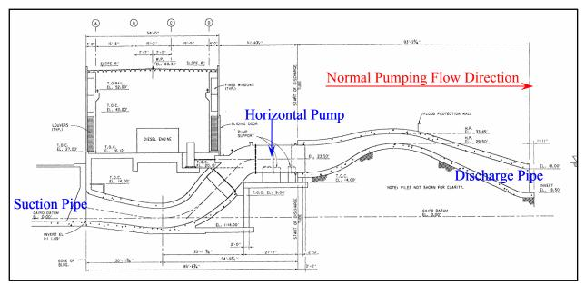
Figure 7-12 – Typical Section through Suction Tube, Horizontal Pump, and Discharge Tube
