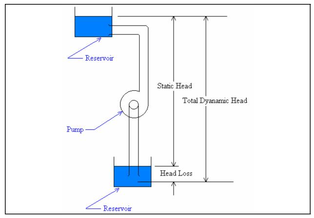
Figure 7-11 shows the relationship between total dynamic head, static head, and head loss.
