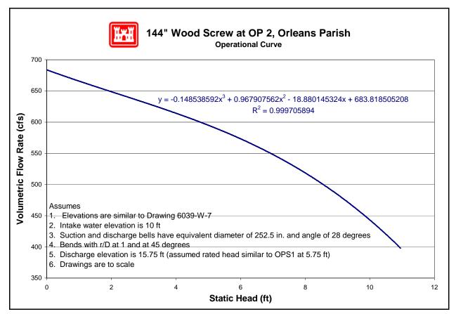
Operational Curve for 144" Wood Screw Pump at OP 2
