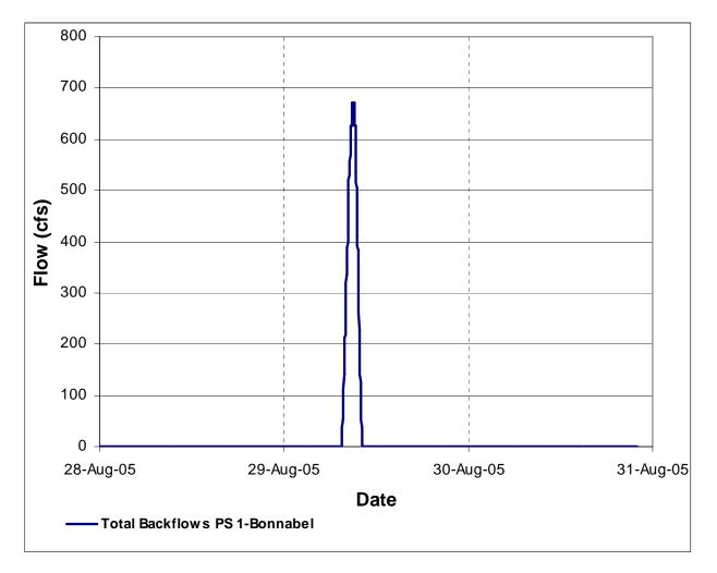
Figure 1-10. Estimated Backflow Hydrograph, East Bank, Bonnabel Pump Station
