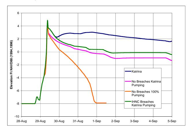
Figure 2-19. Calculated Water-Surface Elevations in Storage Area 2
